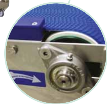
Support and bearing completely in stainless steel machine caption
